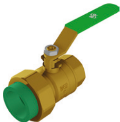
BR PP-RCT Ü-Kugelhahn-Messing IG-zyl verschraubt Runddichtring-EPDM 20°C/1,0MPa grün BR PP-RCT Transition-Ball valve Brass female-thread-cyl with union-nuts O-Ring-gasket-EPDM 20°C/1.0MPa green
